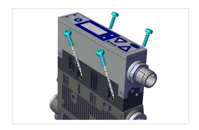
2. Disconnect the vacuum module (1) from the control (2) 1 and remove the compression springs and sealing 2.
