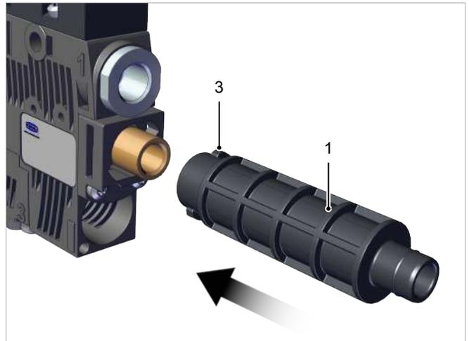
5. Lock the silencer cover (1) by turning the bayonet fastener 90° clockwise (stop).
