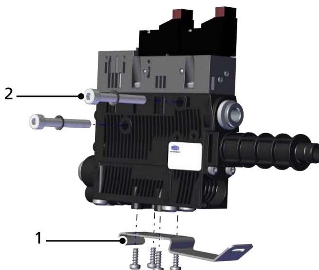
1 DIN rail mount for TS35 DIN rail, incl. plastic tapping screws
