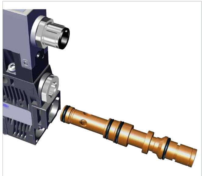
2. Check the nozzle and clean or replace it if necessary.
