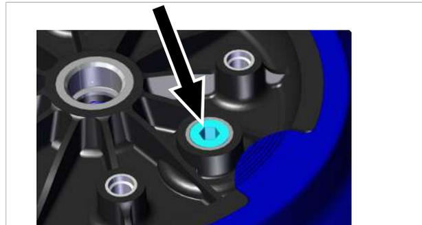
2. For sealing, prepare the male thread in the area displayed on the touch valve with a PTFE strip or low-strength thread lock before mounting.
