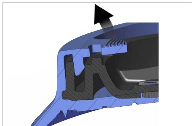
⇒ The sealing ring and suction cup connection disc are detached.
