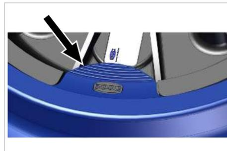
4. Continue pulling the sealing ring from this location over the suction cup connection disc and insert it into the slot until the suction cup connection disc is completely inserted into the sealing ring and the sealing ring does not protrude over the suction cup connection disc at any point, i.e. it must be flush.
