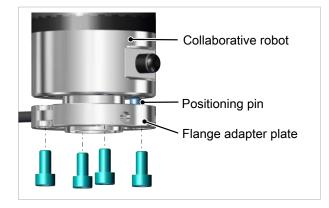
Tightly connect the ECBPMi to the flange adapter plate using the bayonet fastener. Position the ECBPMi so that the small triangle points toward the groove on the flange adapter plate.
