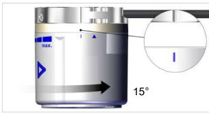
4. NOTE! End position is not reached and the line on the ECBPMi does not match the groove on the flange. Screwing in the locking screws damages the light conductors. They are then secured against being opened unintentionally with the two screws (M3x14). Observe the max. tightening torque of 0.6 Nm.
