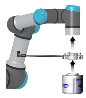
Position the flange adapter plate included in the delivery on the suitable collaborative robot using the positioning pin and fasten it using the four M6x12 cylinder head screws. Observe the permitted tightening torque for the thread.
