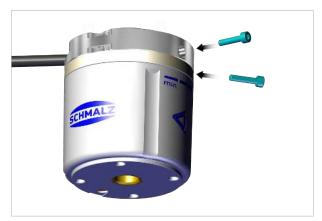
To attach the vacuum suction cup, vacuum end effector or custom gripper:
