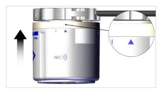
3. Turn the ECBPMi clockwise by 15° (until it stops) (the line marking matches the groove on the adapter flange).
