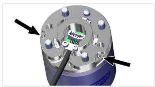
The electrical interface to the robot is customer-specific. The PIN assignment on the flange connector (1) is always the same.
