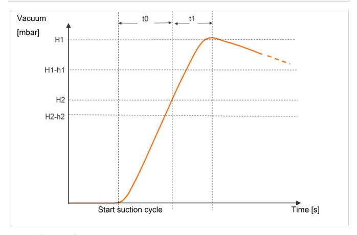
The specified value for the max. permitted evacuation time t1 can be set using the IO-Link ("Permissible evacuation time" parameter) [0x006B]. Setting the value to "0" (= off) deactivates monitoring. The maximum permitted evacuation time setting is 9.99 s.
