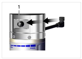
2. Optional: Use cable ties to fasten the connection cable to the drilled holes on the flange so that it is laid tightly against the robot arm.
