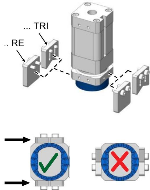
**Important:** Only the Schmalz holder system (accessories) may be used for the lateral connection.
