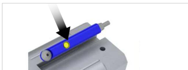
2. Push the sensor to the stop of the T-slot, or in the case of variants with **open T-slot**, fix the sensor flush with the lower end of the slot (towards the gripping surface).
