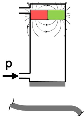
The bistable mode of operation allows safe gripping even during a power failure.
