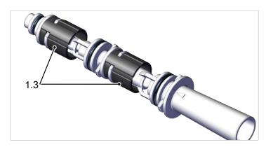
5. Grease the O-rings slightly before mounting the ejector module.
