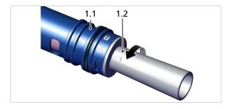
2. Pull the nozzle fitting (1.2) out of the main body (1.1) using only axial forces.
